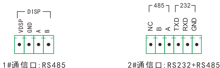
Figure 4.10 Schematic diagram of two communication interfaces of the instrument
